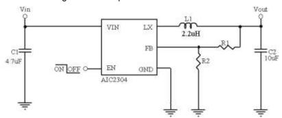
Fig. 2 Adjustable Step-Down DC/DC Converter
