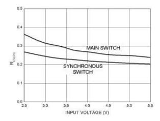
Fig. 7 R<sub>DS(ON)</sub> vs. Input Voltage
