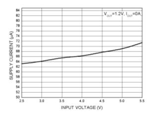
Fig. 8 Supply Current vs. Input Voltage
