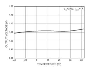
Fig. 10 Output Voltage vs. Temperature
