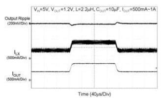
Fig. 15 Load Transient Response
