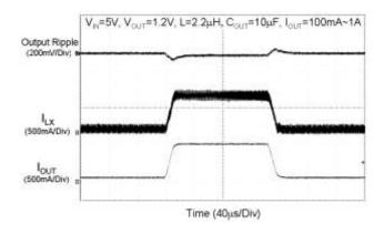
Fig. 13 Load Transient Response
