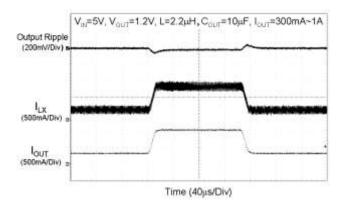
Fig. 14 Load Transient Response
