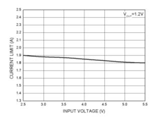
Fig. 9 Current Limit vs. Input Voltage
