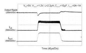
Fig. 11 Load Transient Response
