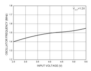
Fig. 6 Oscillator Frequency vs. Input Voltage
