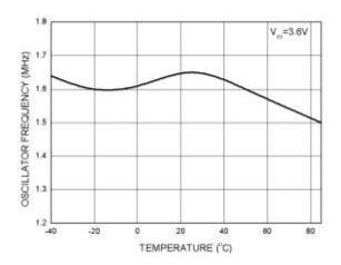
Fig. 5 Oscillator Frequency vs. Temperature
