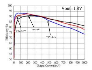
Fig. 3 Efficiency vs. Input Voltage
