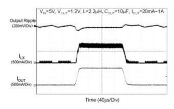
Fig. 12 Load Transient Response
